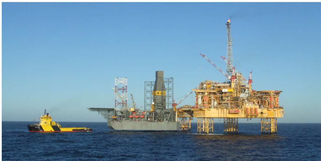
THE ROWAN GORILLA V. The rig is about to enter the water alongside the Elgin WHP, with the Vidar Viking on the tow. Picture: Crew of the Island Pride.
