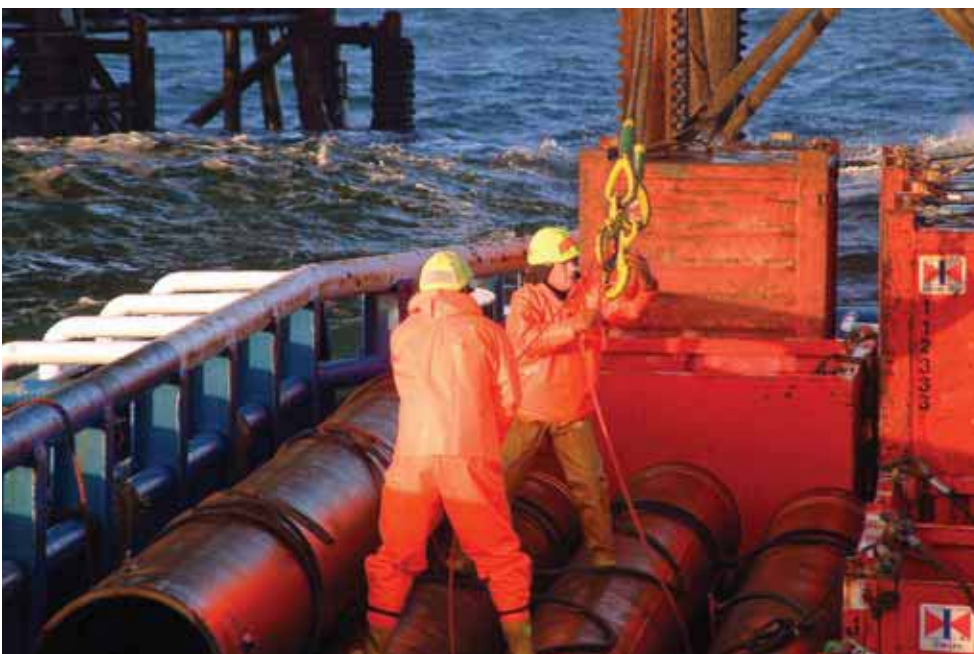
Casing being discharged at a jack-up. Over the duration of a drilling programme thousands of feet of tubulars will be discharged to the rig. Picture: David Styles.
