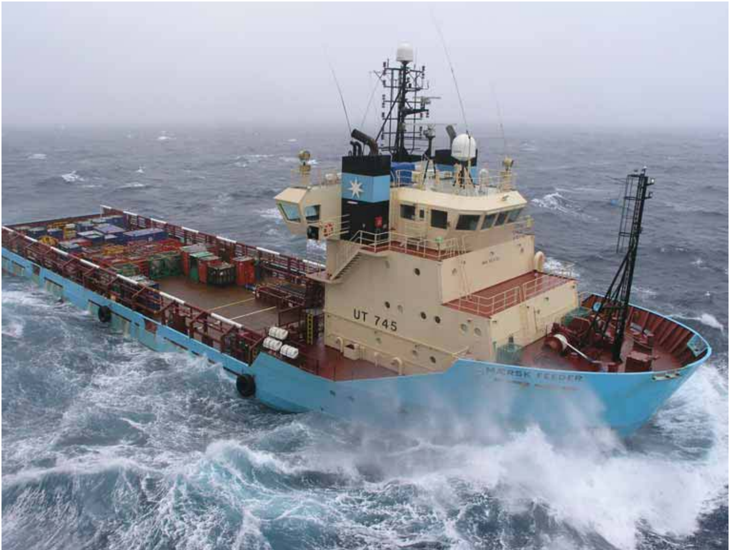
The UT745 Maersk Feeder at an offshore installation. Modern platform ships can remain in position in weather which prevents the offshore cranes from operating. Picture: Victor Gibson.
